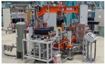
Kobe already has a strong position in the world of tire uniformity machines, but it has now begun selling the Librota-GS. Kobe claims the new model has the world's fastest cycle time of 18 seconds per tire and the world's highest repeated measurement accuracy. Kobe claims the new Librota-GS has achieved a repeated measurement accuracy of 1.69N or lower, compared with conventional machines of 2.40N or lower.
